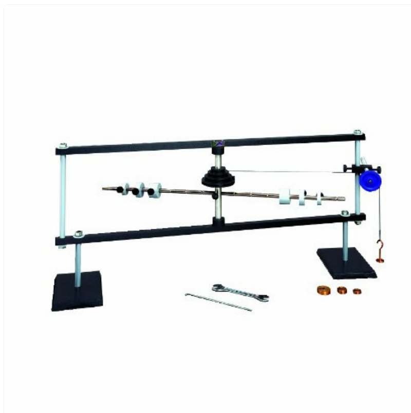
Figure 1: Fully assembled 3B Scientific U29385 Economy Rotation Apparatus, showing the main frame, rotating rod with counterweights,
