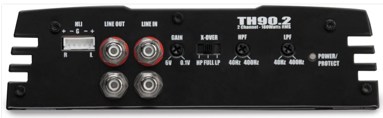
Figure 5: View of the input and control panel on the MTX Audio TH90.2 amplifier. This image displays the HLI (High-Level Input) connector, LINE OUT and LINE IN RCA jacks, GAIN control, X-OVER switch (HP, FULL, LP), HPF and LPF adjustment knobs, and the POWER/PROTECT indicator light.
