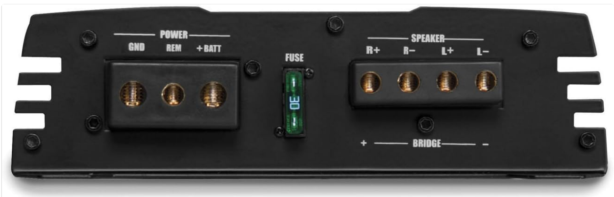
Figure 4: View of the power and speaker terminal block on the MTX Audio TH90.2 amplifier. This image clearly shows the GND, REM, +BATT terminals, the fuse slot, and the SPEAKER output terminals (R+, R-, L+, L-), along with the BRIDGE connection points.
