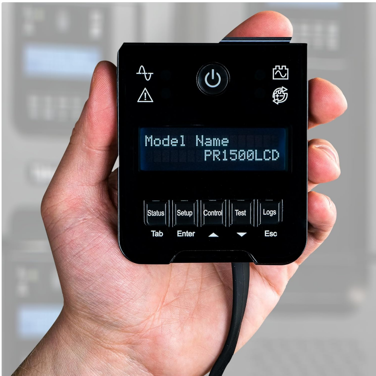
Figure 3: The detachable LCD panel of the CyberPower PR1500LCD is shown being held, demonstrating its portability and ease of remote monitoring.
