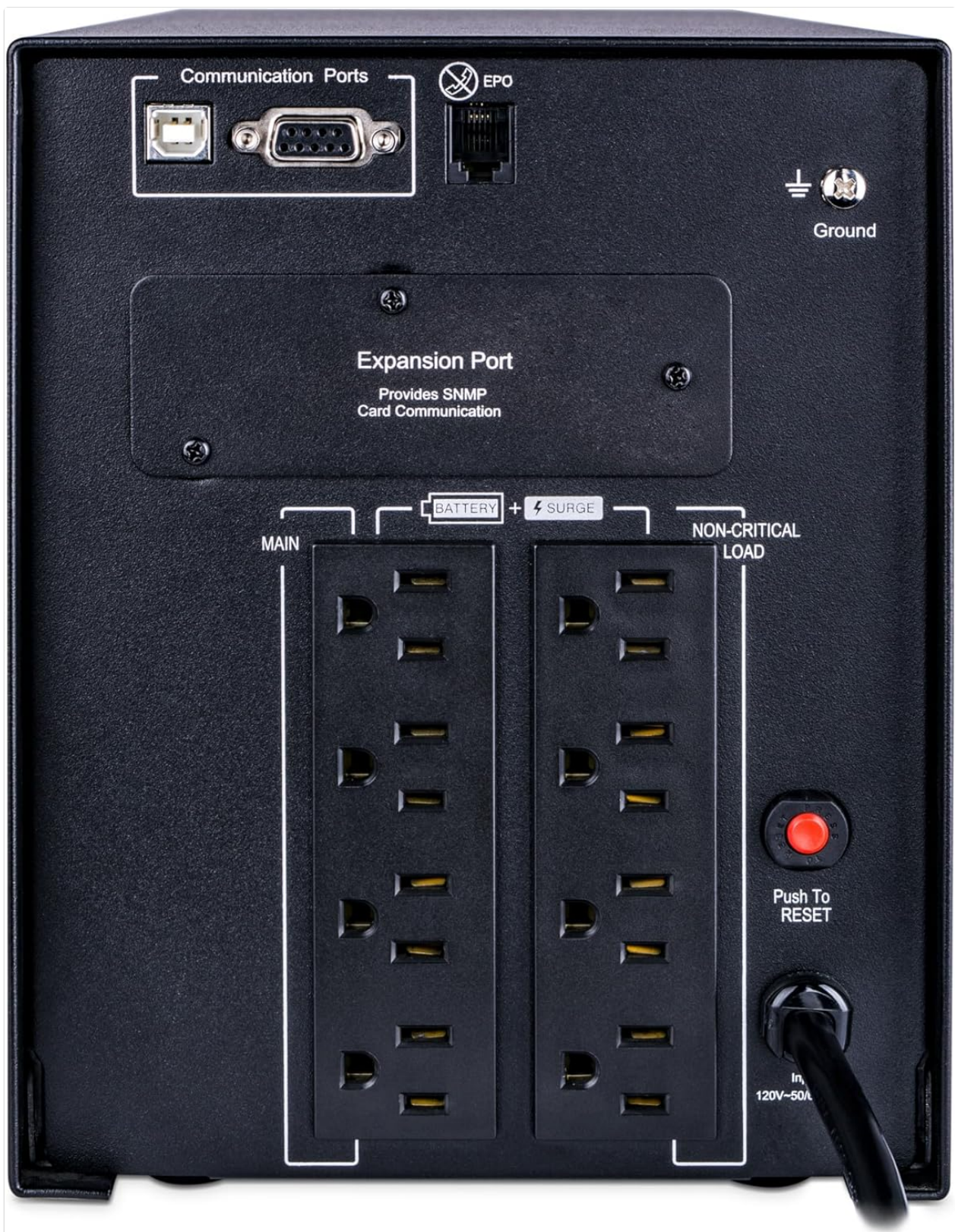
Figure 4: The rear panel of the CyberPower PR1500LCD, displaying communication ports (USB, Serial, Network), an expansion port for SNMP card communication, and the NEMA 5-15R outlets, clearly labeled for battery/surge protected and surge-only connections. A circuit breaker reset button is also visible.
