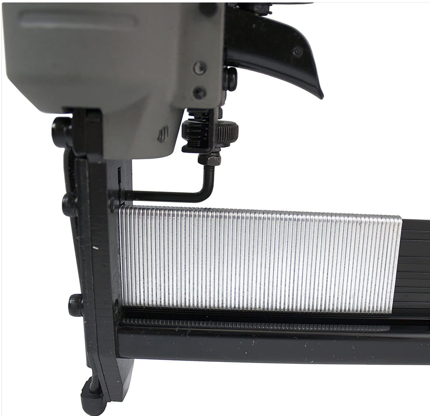
Figure 5.2: A strip of brad nails correctly loaded into the tool's magazine.
