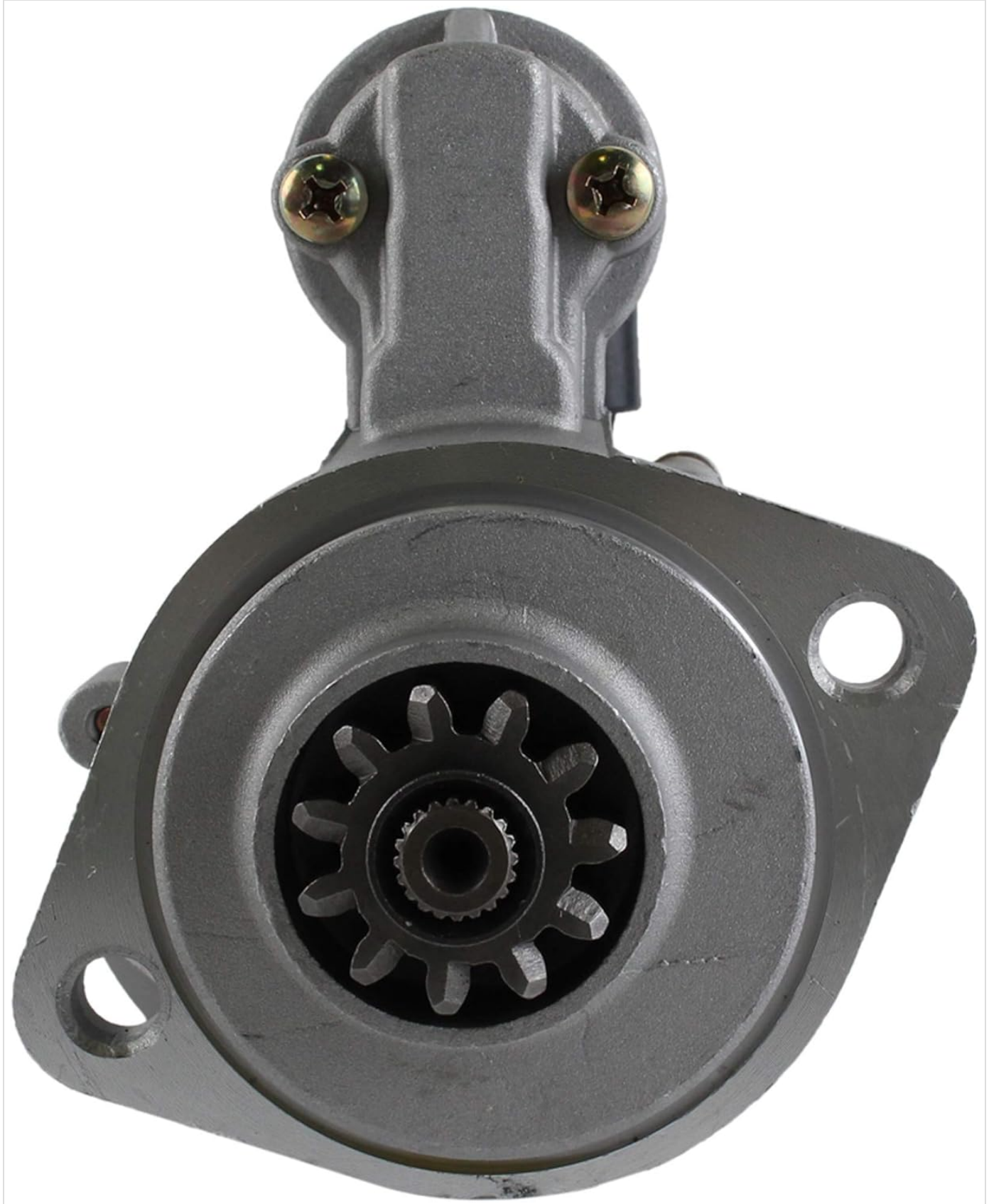
Figure 4: Close-up view of the starter's drive gear (bendix). Inspect this area for wear or damage if the starter spins but does not engage the engine.
