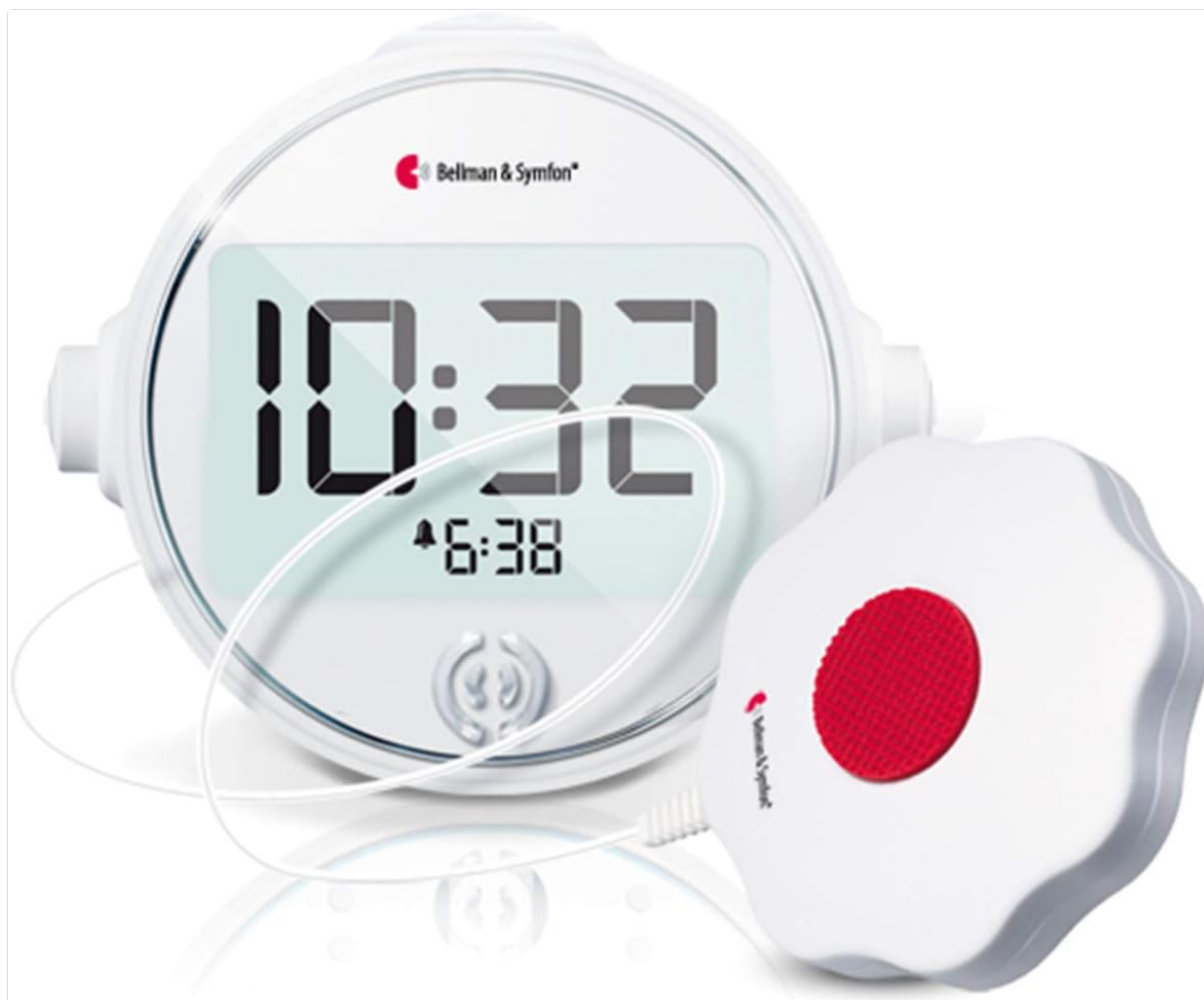
Figure 3.1: Bellman & Symfon Alarm Clock Classic (BE1350) main unit and connected bed shaker.
