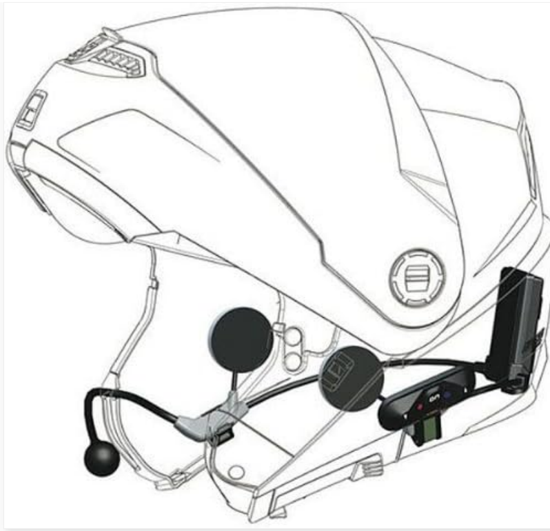
Figure 3: Detailed view of the N-COM B4 system components, including speakers, microphone, and control unit, integrated into a helmet.
