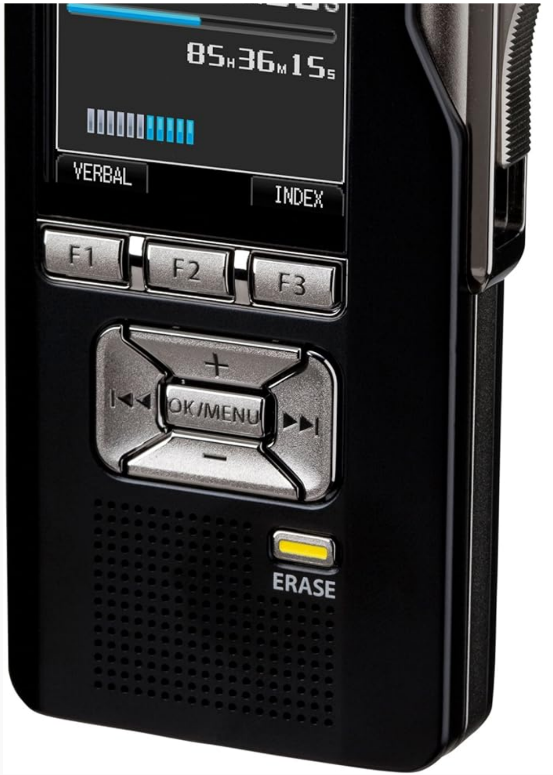
Figure 2.1: Front view of the Olympus DS-7000 Digital Voice Recorder, showing the display, function buttons, navigation controls, and microphone.
