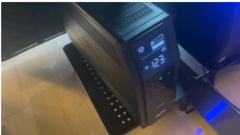
Close-up of the APC SMC1000 Smart-UPS LCD display, showing current voltage, load, and battery charge level.
