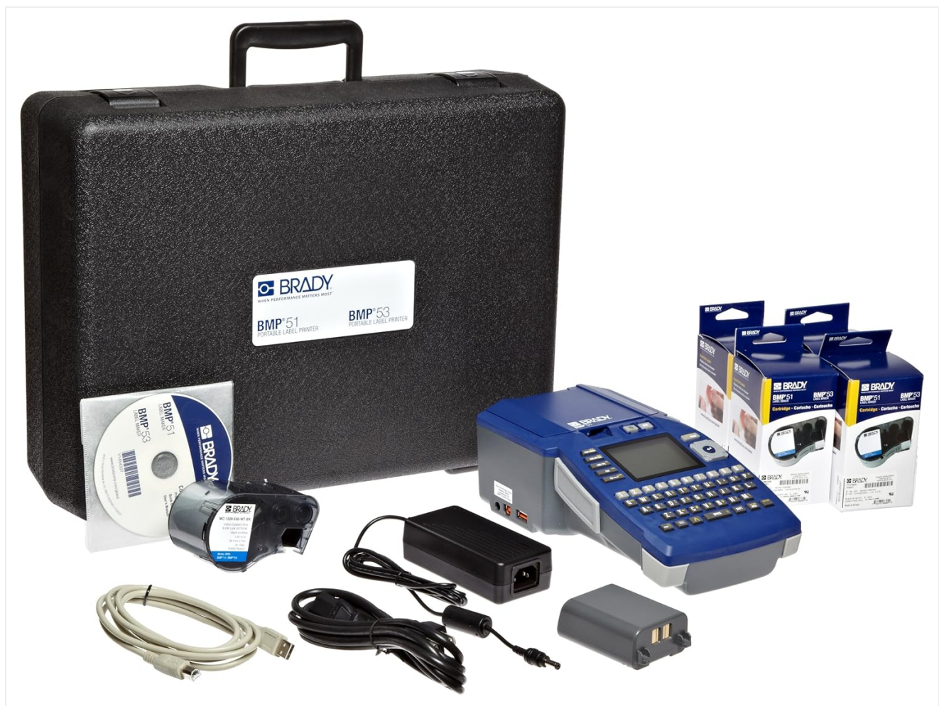
Figure 2.1: All components included in the Brady BMP51 Voice and Data Communications Starter Kit, including the printer, hardcase, cables, power adapter, battery, and various label cartridges.
