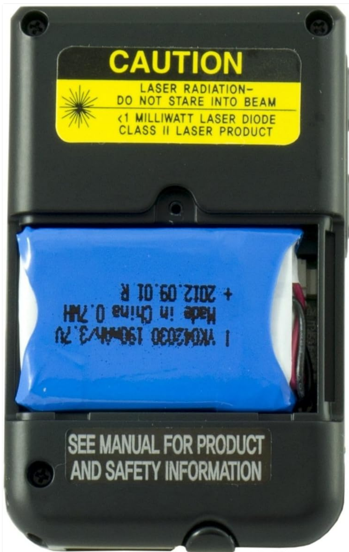
Image: The KDC20/100/200 190mAh battery installed in a compatible device. Note the caution label on the device indicating "LASER RADIATION - DO NOT STARE INTO BEAM" for devices with laser components. This image highlights the proper placement of the battery within the device's battery compartment.
