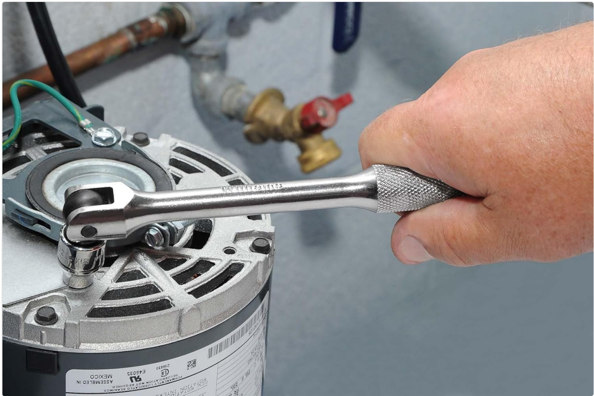
Figure 3: Proper attachment and use of a socket with a ratchet on a fastener.
