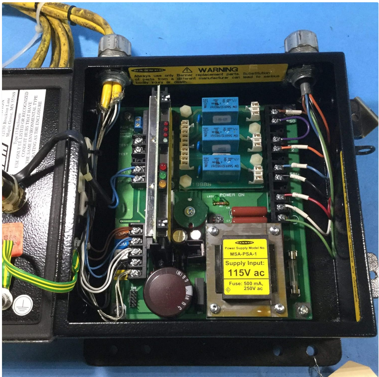
Figure 3.2: Internal components of the MSCA-1 Control Box, including the main circuit board and power supply.
