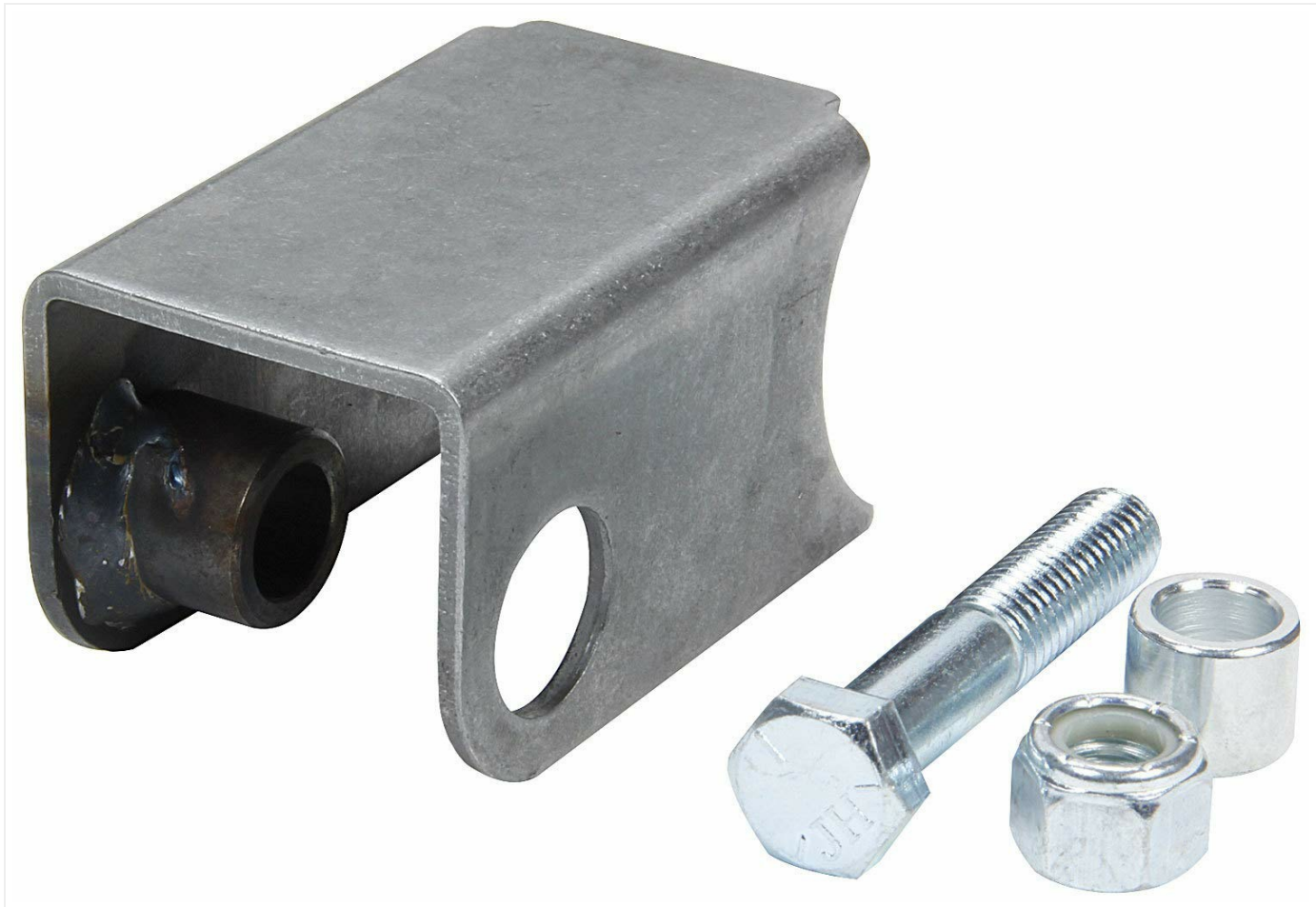
Figure 1: The Allstar Performance ALL60104-10 Coil-Over Bracket, shown with the included mounting bolt, locknut, and spacer. The bracket features a notched design for welding to round tubing and a pre-drilled hole for the bolt.
