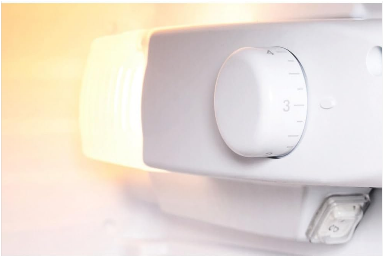
A detailed shot of the internal thermostat dial, used to adjust the temperature settings of the refrigerator, located near the interior light.
