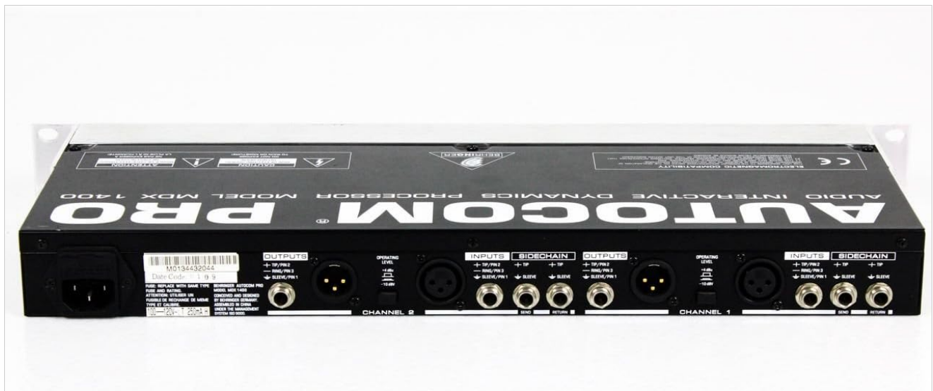
Figure 3.2.1: Rear panel connections of the MDX1400. This image displays the XLR and 1/4" TRS jack inputs, outputs, and sidechain connections for both channels, along with the power inlet.
