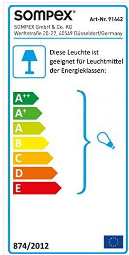
Figure 3: Energy Efficiency Label for Sompex Toledo 91442. This label indicates that the luminaire is suitable for light sources of energy classes A++ to E, according to regulation 874/2012.
