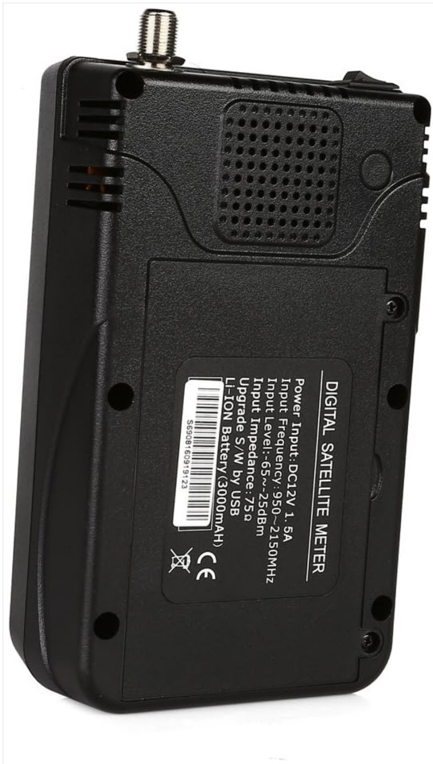
Image 3: Rear view of the Satlink WS-6908 SE, showing the speaker grille and battery cover.
