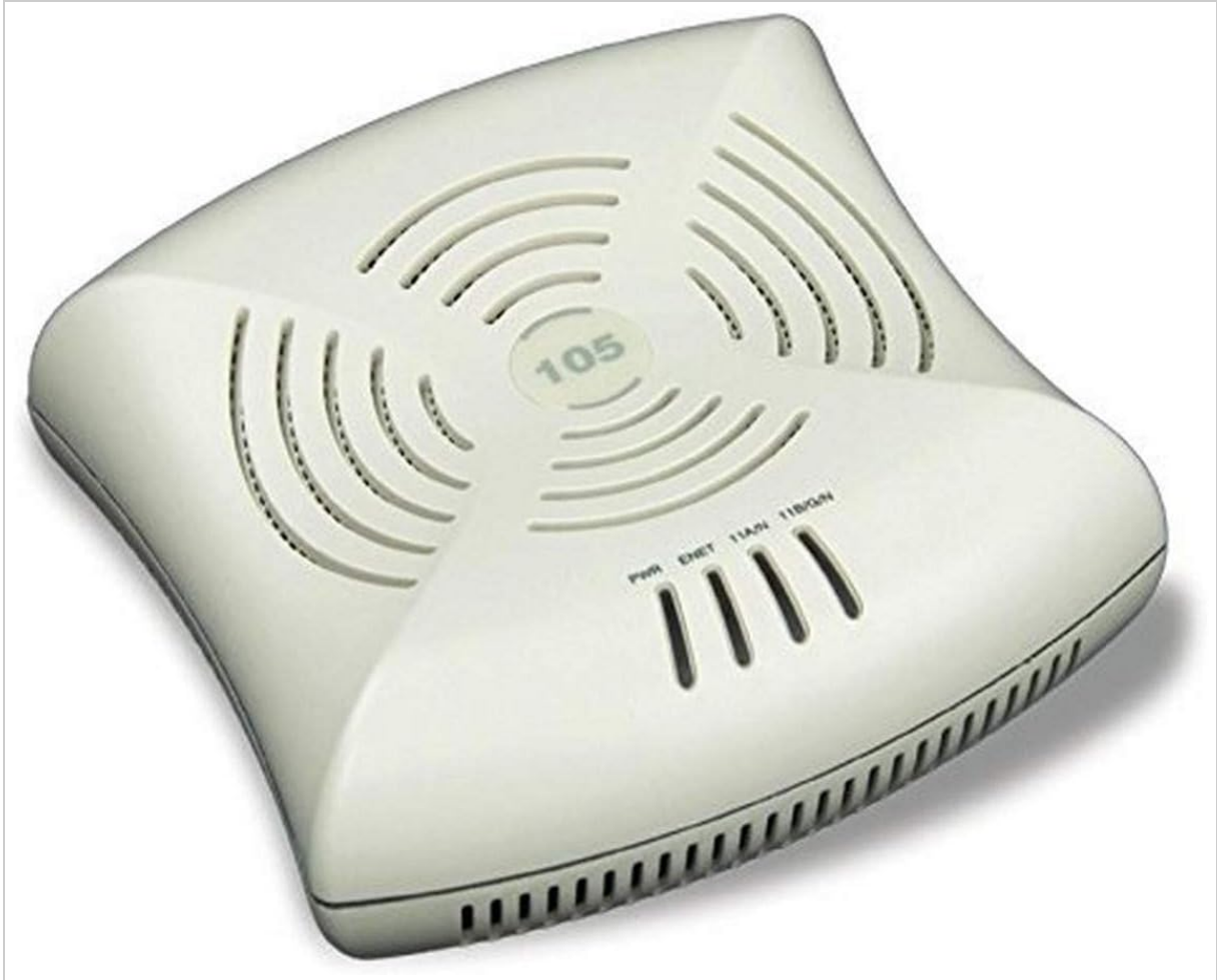
Image: The Aruba AP-105 Wireless Access Point. This image shows the top view of the access point, highlighting its compact design, ventilation grilles, and LED indicators for Power, Ethernet, 11AN, and 11BGN connectivity. The model number "105" is visible in the center.
