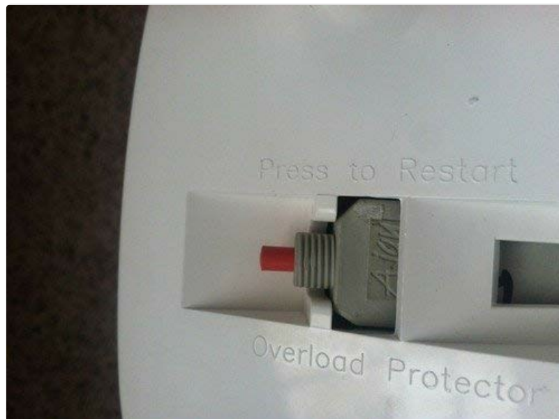
Image: A close-up view of the red reset button, labeled 'Press to Restart Overload Protector', located on the underside of the mixer grinder unit.
