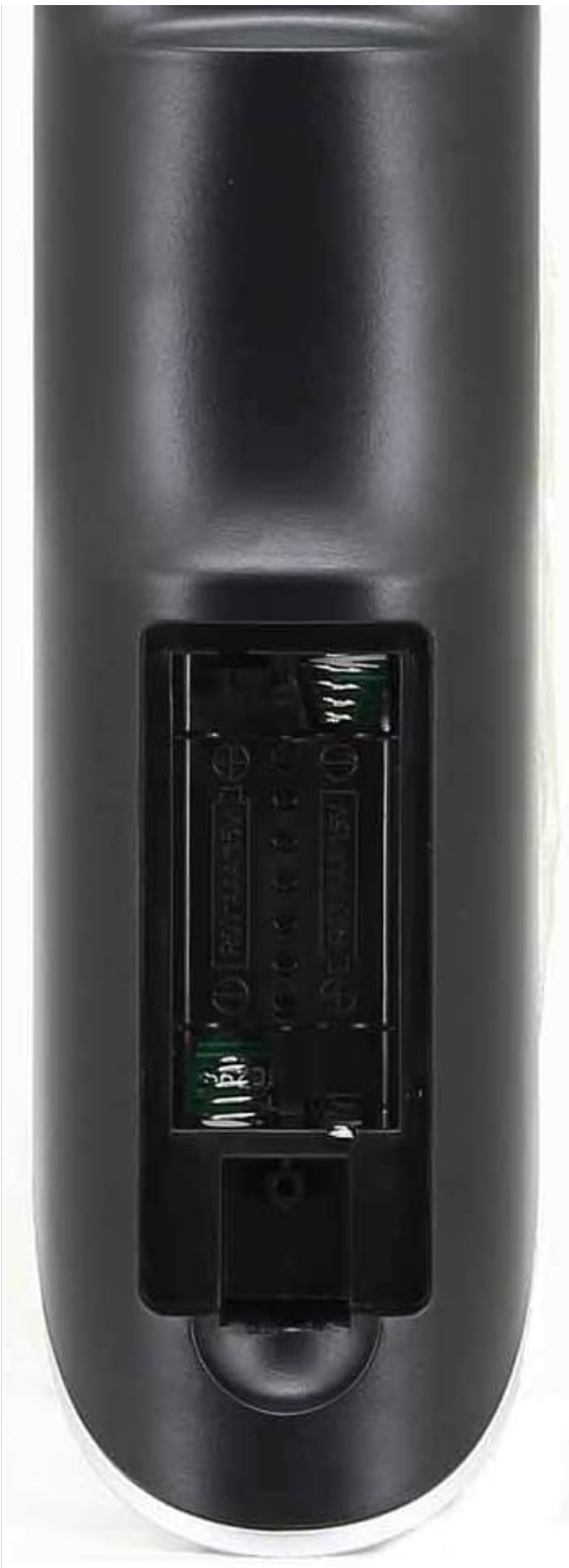
Figure 2.4: Rear view of the remote control with the battery cover removed, illustrating the two AAA battery slots.
