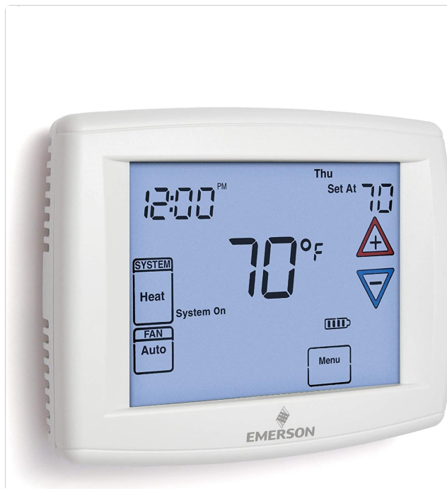
Figure 1: Main display of the Emerson 1F95-1291 Touchscreen Thermostat. It shows the current time (12:00 PM), day (Thursday), actual room temperature (70°F), and the set temperature (70°). The system is in "Heat" mode and the fan is set to "Auto". A "Menu" button is visible for accessing settings.
