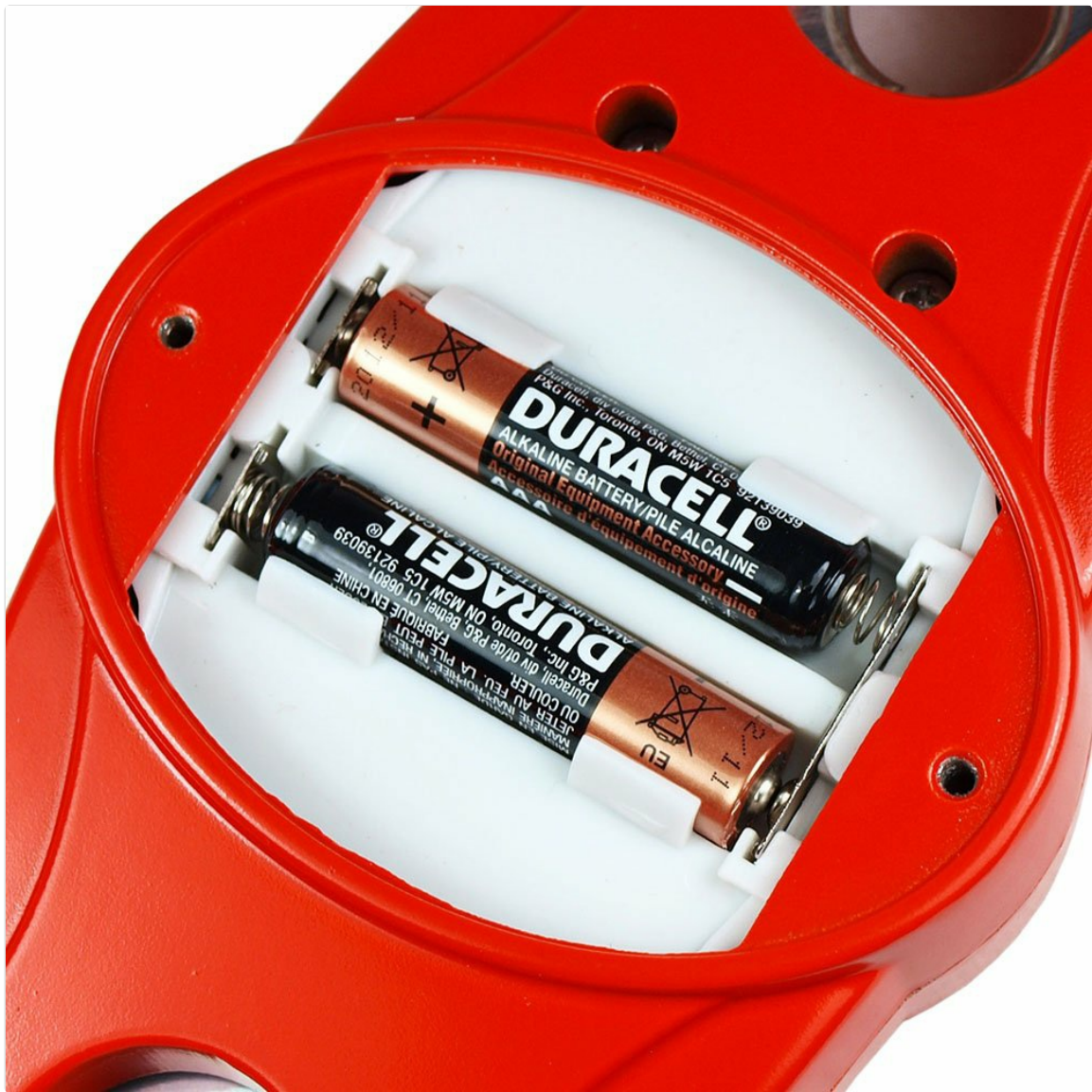
Image: A detailed view of the battery compartment, showing the correct placement of two AAA batteries.
