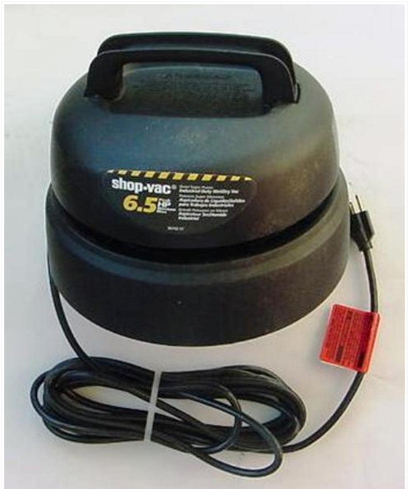
Image 1: The Shop-Vac Service Power Unit, showing the motor housing, handle, and coiled power cord with a red warning tag.
