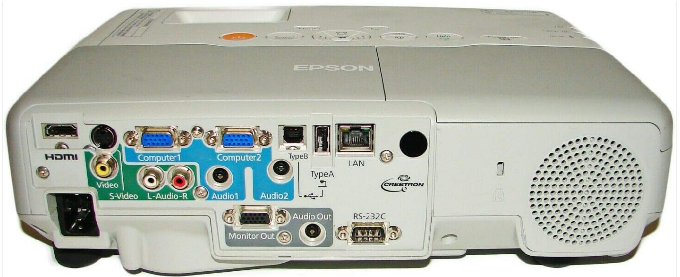
Image: Rear view of the projector displaying various input and output ports, including HDMI, VGA (Computer1, Computer2, Monitor Out), S-Video, Composite Video, Audio In/Out, USB (Type A, Type B), LAN (RJ-45), and RS-232C.
