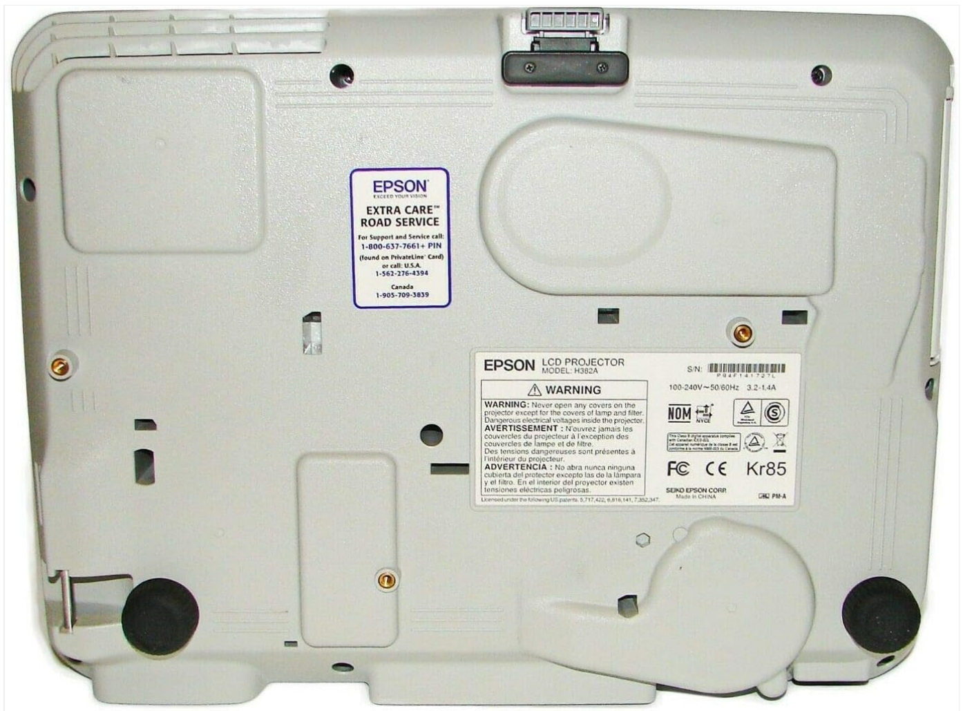
Image: Bottom view of the projector, showing mounting points, adjustable feet, and product information labels including serial number and electrical ratings.
