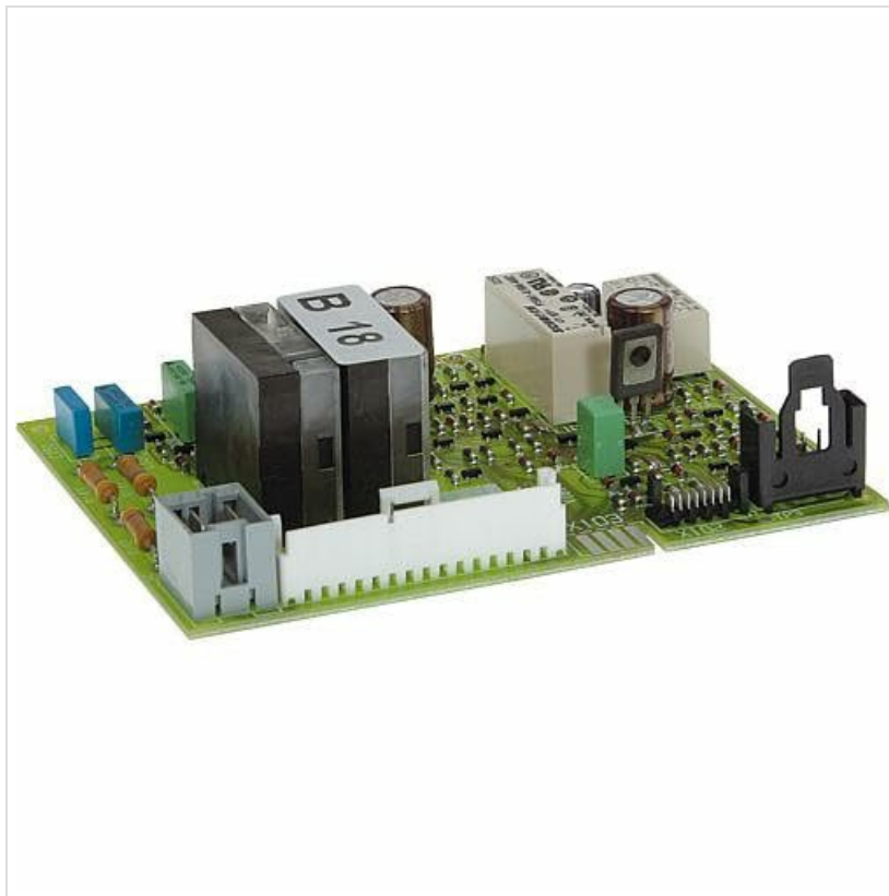
Figure 1: Vaillant 100547 Automatic Gas Igniter. This image displays the circuit board with various electronic components, including relays, resistors, and connectors, which collectively manage the ignition process.
