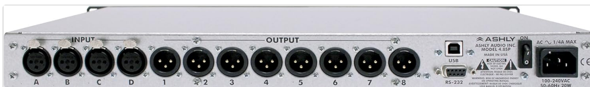
Figure 2: Rear view of the Ashly Protea 4.8SP, showing balanced XLR inputs (A, B, C, D), balanced XLR outputs (1-8), USB port, RS-232 port, and AC power inlet.
