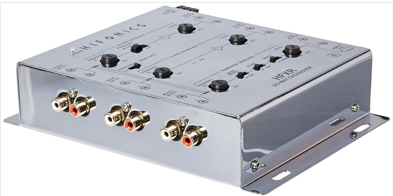
Figure 3: Top view of the HFXR Crossover, highlighting the frequency, level, and mode adjustment knobs.
