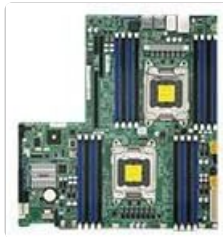
Figure 1: Overview of the Supermicro X9DRW-3F Motherboard. This image displays the main components including CPU sockets, RAM slots, and various connectors.
