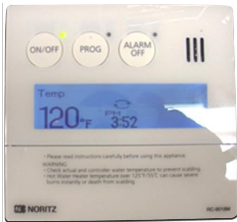
Figure 1: Noritz RC-9018M Commercial Remote Controller. The display shows the current temperature (120°F) and time (3:52 PM). Control buttons include ON/OFF, PROG (Program), and ALARM OFF. A warning about scalding is visible at the bottom.
