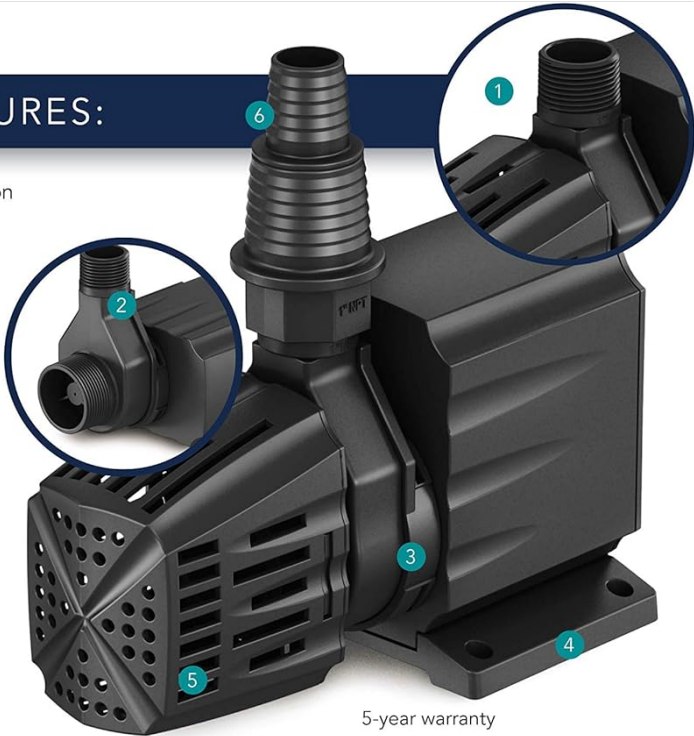
Image: Diagram highlighting key features of the MD-Series pump, including oversized male threaded inlet/outlet, rotating volute, removable stable base, and removable pre-filter. It also notes the 5-year warranty.
