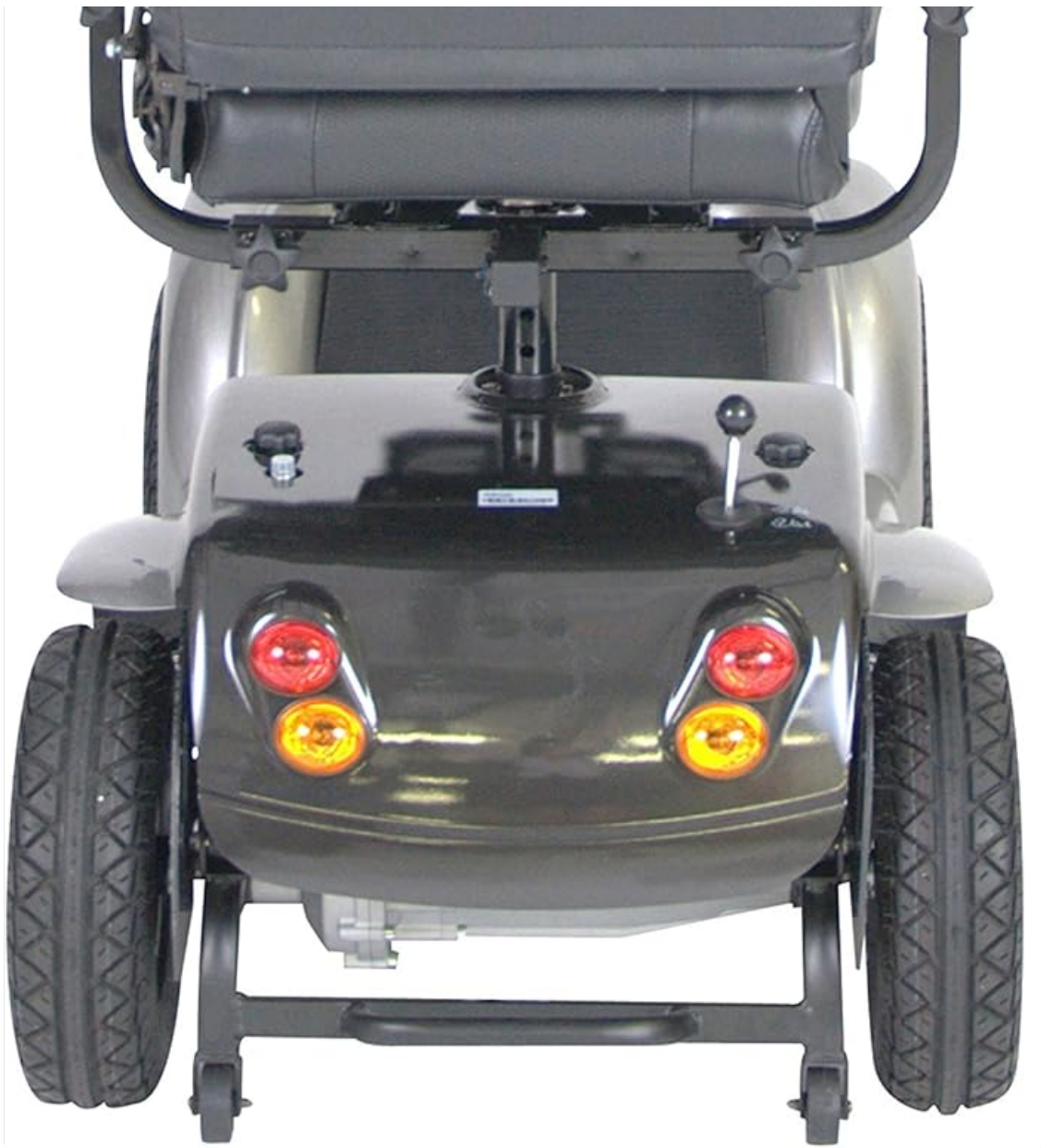
Figure 4: Rear view of the scooter, displaying the tail lights and anti-tip wheels.
