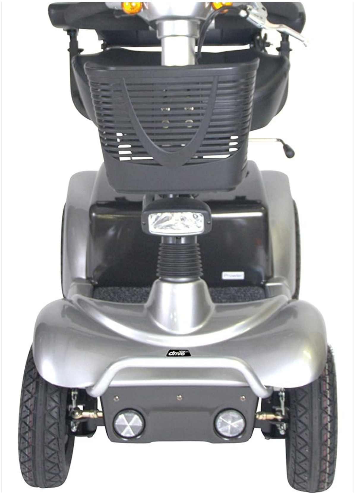
Figure 2: Front view of the scooter, highlighting the headlight, turn signals, and front basket.
