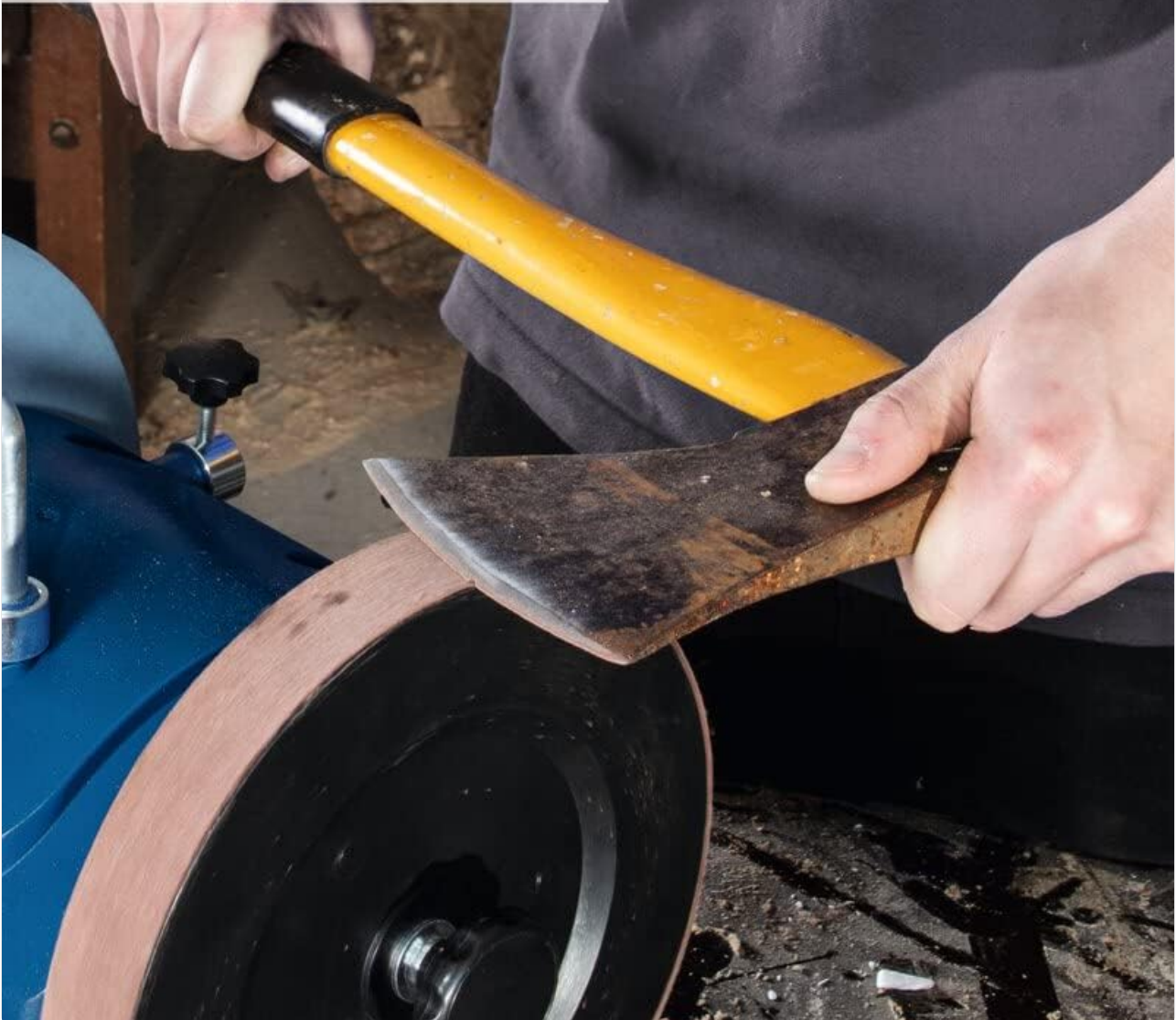
Image: A user demonstrating the deburring process on the Tiger 2000S, using the leather honing disc to remove the burr from an axe blade and achieve a perfect cutting edge.
