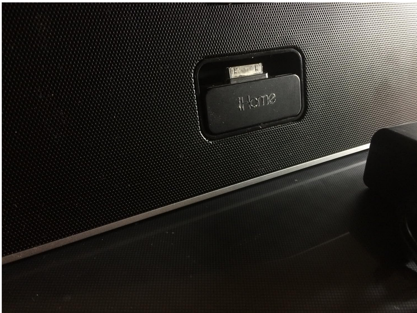
Figure 2: A detailed view of the 30-pin dock connector on the iHome iD7SC, ready to receive an Apple device.
