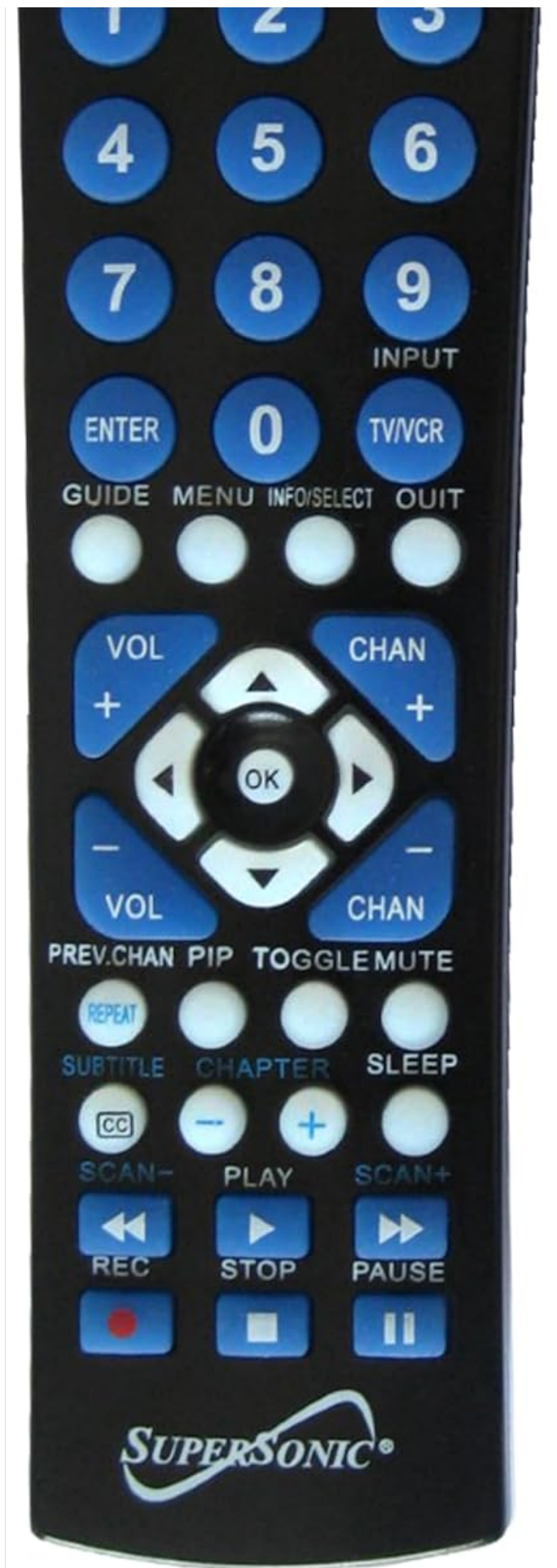
Image: Front view of the Supersonic SC-26 Universal Remote Control, showcasing its layout with large, blue and white buttons for numbers, channel, volume, and device selection.
