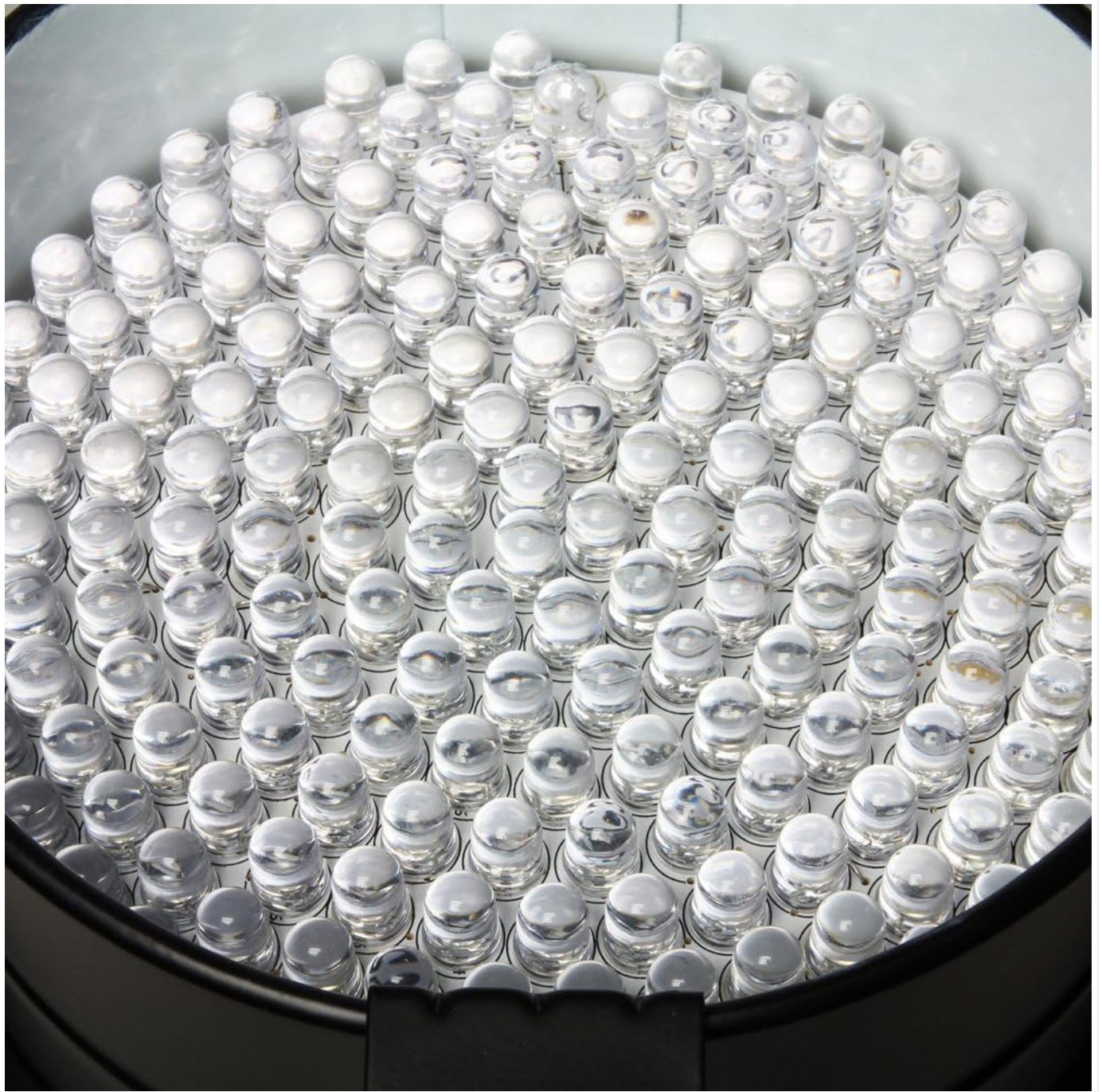
Figure 4.4: Detailed view of the 10mm LED array, highlighting the individual red, green, and blue diodes.
