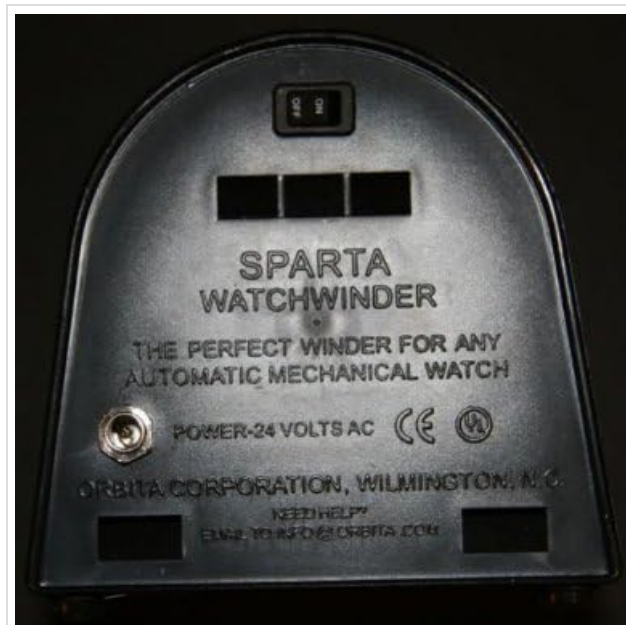
Image: The back panel of the watch winder, clearly showing the ON/OFF toggle switch at the top and the power input jack below.
