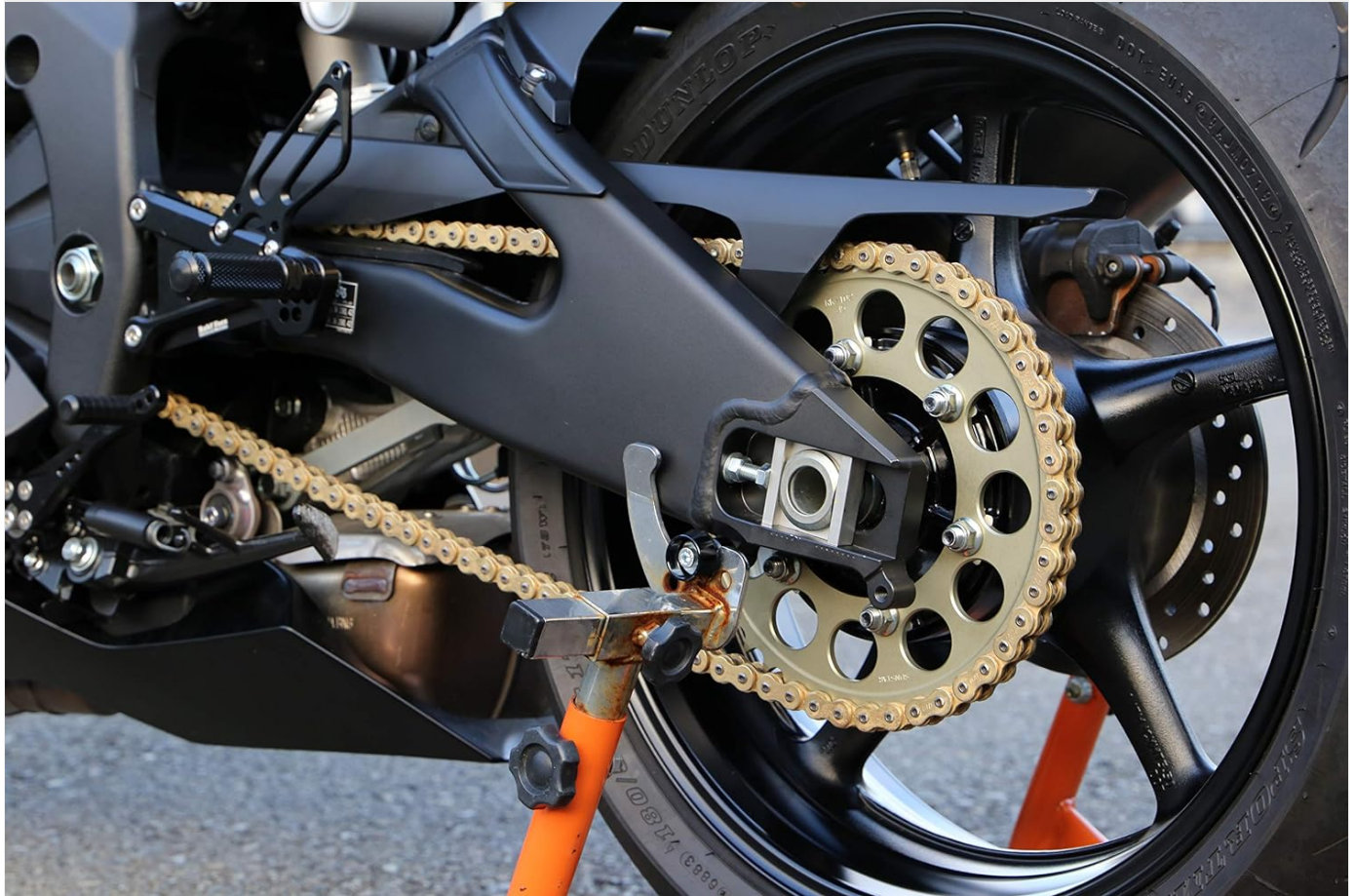
Figure 2: The SUNSTAR rear sprocket installed on a motorcycle. This image shows the sprocket mounted on the rear wheel, connected to the drive chain, illustrating a typical installation scenario.
