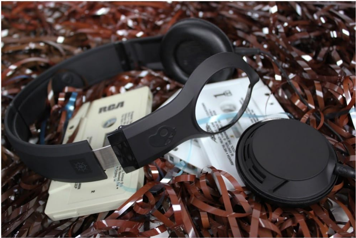
Figure 3.2: Detached earcup, highlighting the removable design for accessory integration.
