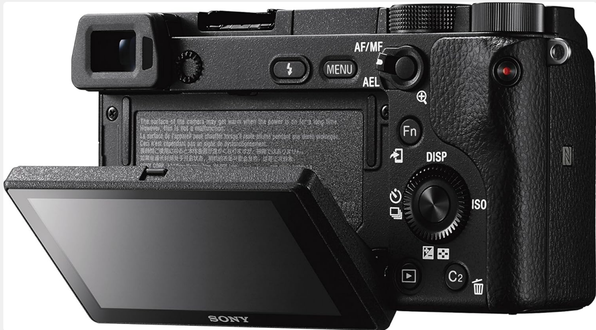
Tilting LCD Screen (Down): The LCD screen tilted downwards, useful for shooting from high angles.
