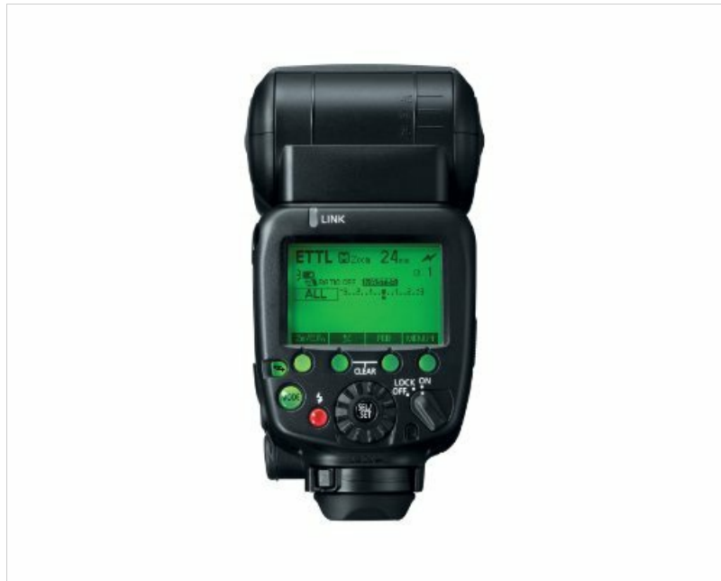
Image 3.2: The LCD panel showing E-TTL mode and zoom settings.
