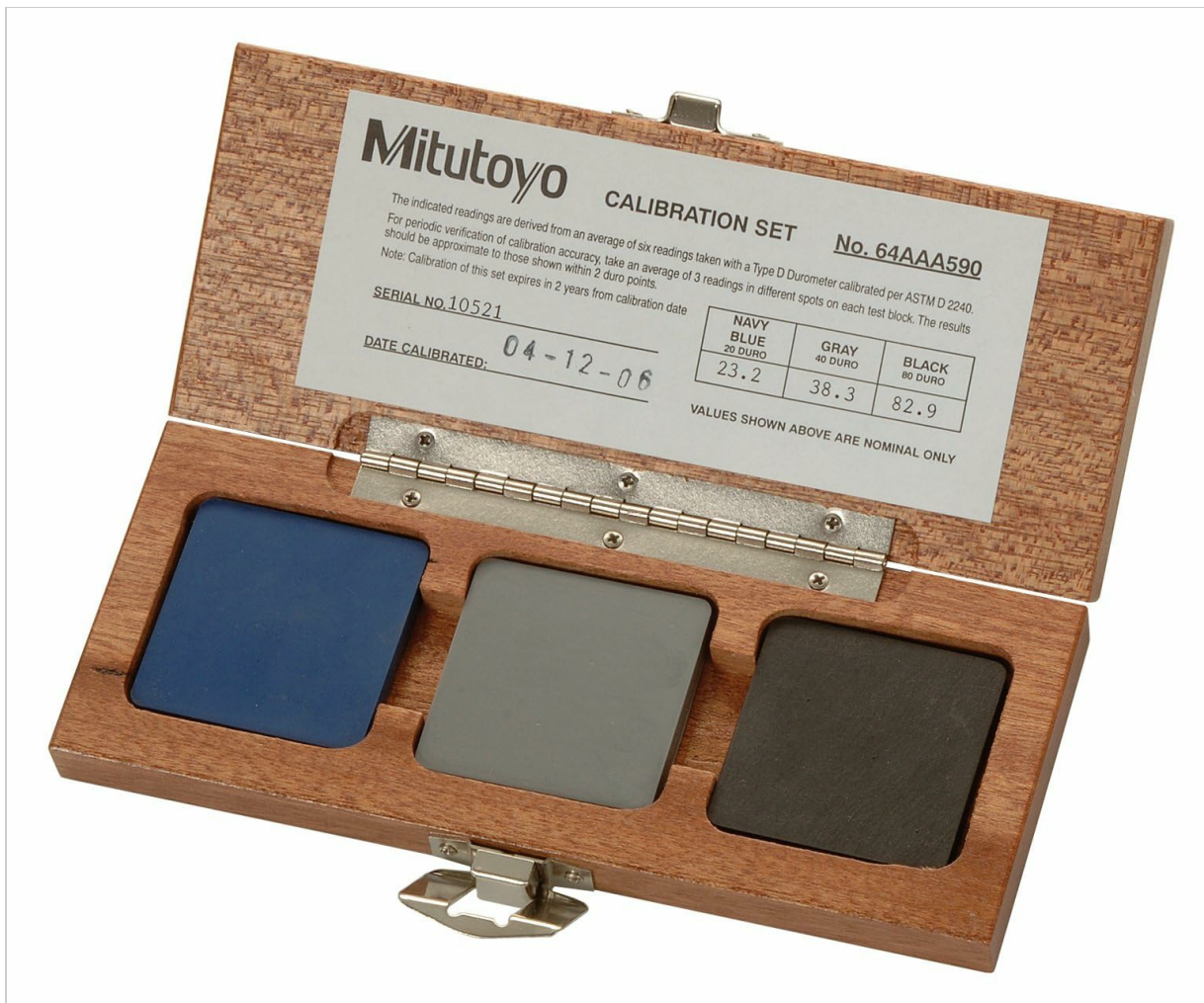
Image 1: Mitutoyo 64AAA590 Calibration Set. The set includes three calibration blocks (blue, gray, black) within a mahogany case. A label inside the lid provides calibration details, including serial number (e.g., 10906), date calibrated (e.g., 10/09/12), and nominal durometer values for each block (e.g., Navy Blue 20 Duro: 21.7, Gray 40 Duro: 34.3, Black 80 Duro: 80.3). Values shown are nominal only.
