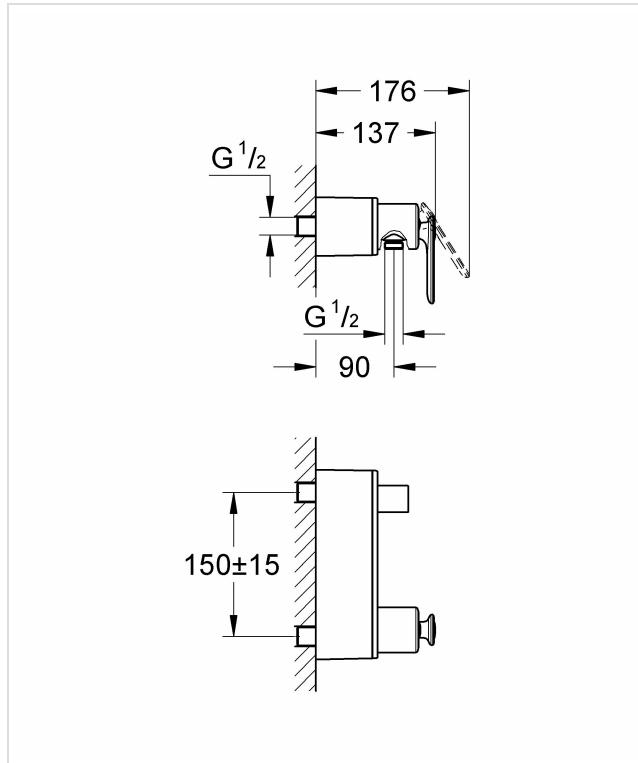
*This technical drawing provides key installation dimensions for the GROHE Veris Shower Mixer. It shows a wall-mount installation with G 1/2 connections, a center-to-center distance of  $150 \pm 15$  mm for the wall connections, and an overall width of 176 mm.*
