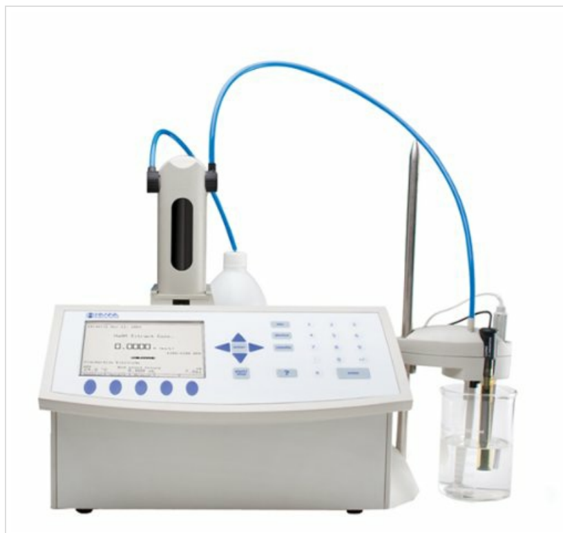
Image of the Hanna Instruments HI 901-01Z Potentiometric Titrator, showing the main unit, the burette driver assembly with tubing, and a beaker with an electrode.
