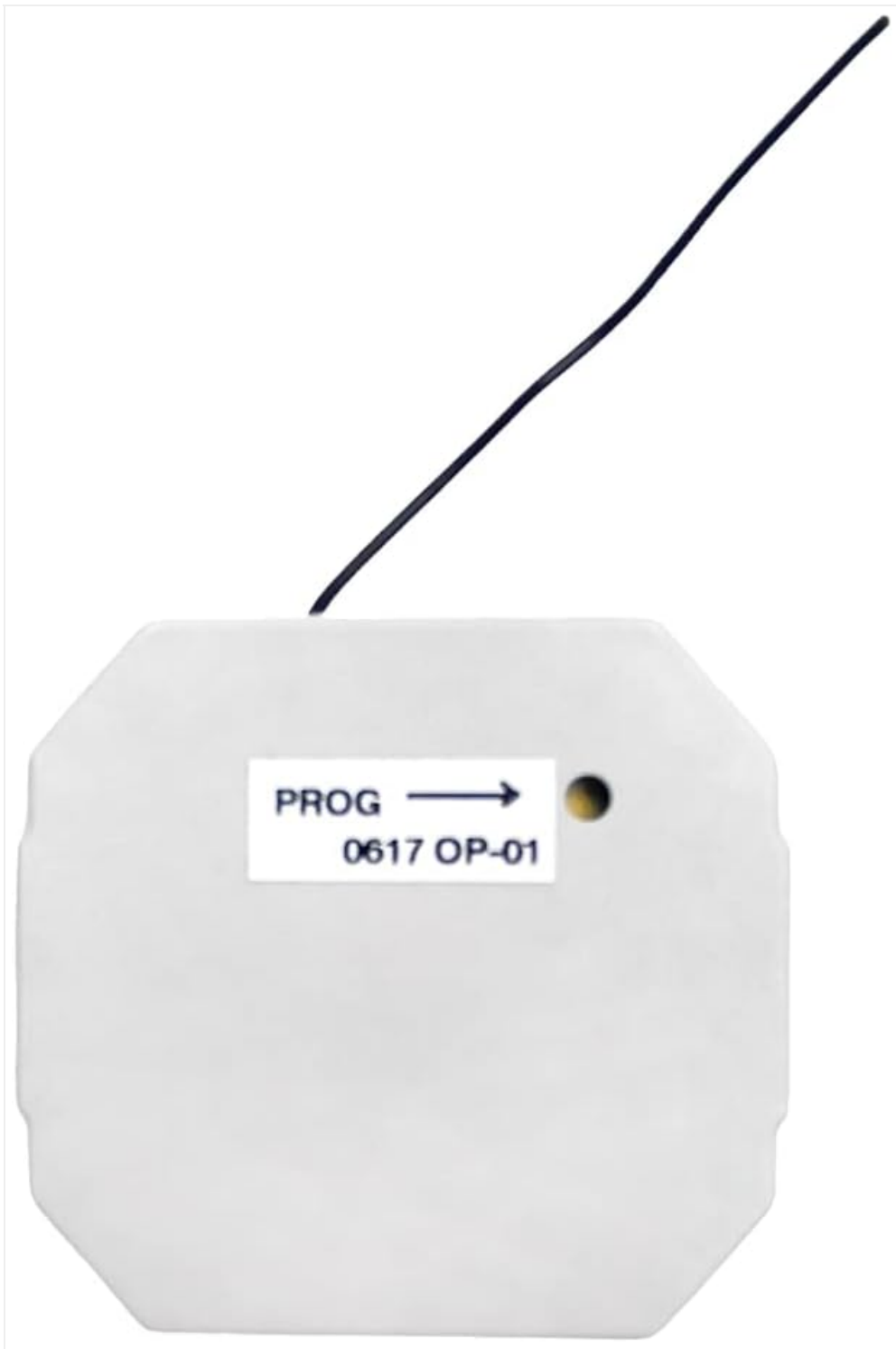
Figure 3.5: Bottom view of the Selve i-R Receive, showing the "PROG" label and button.
