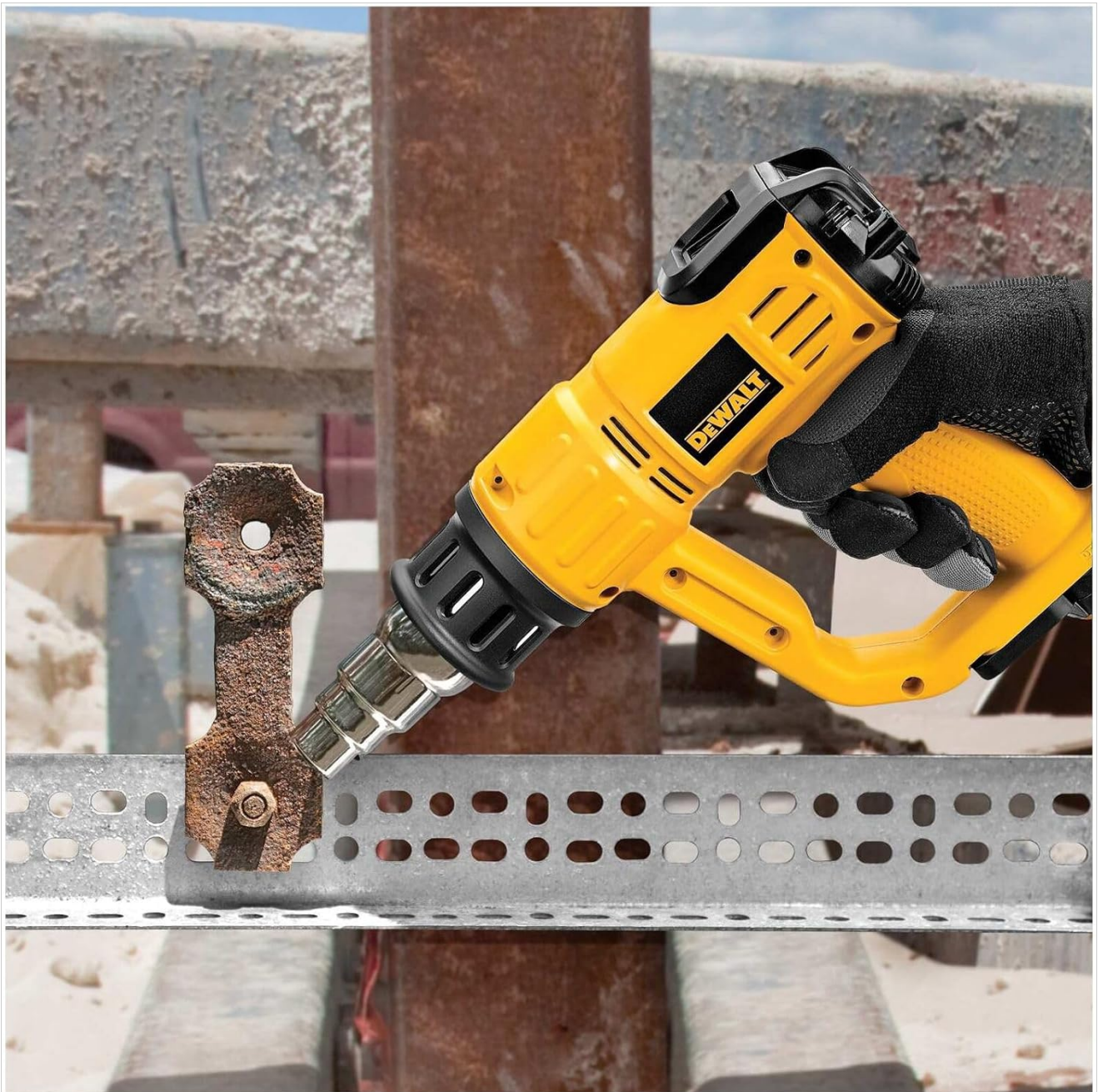
Image: The DEWALT heat gun being used to heat a rusted metal part, illustrating its effectiveness in loosening seized components.
