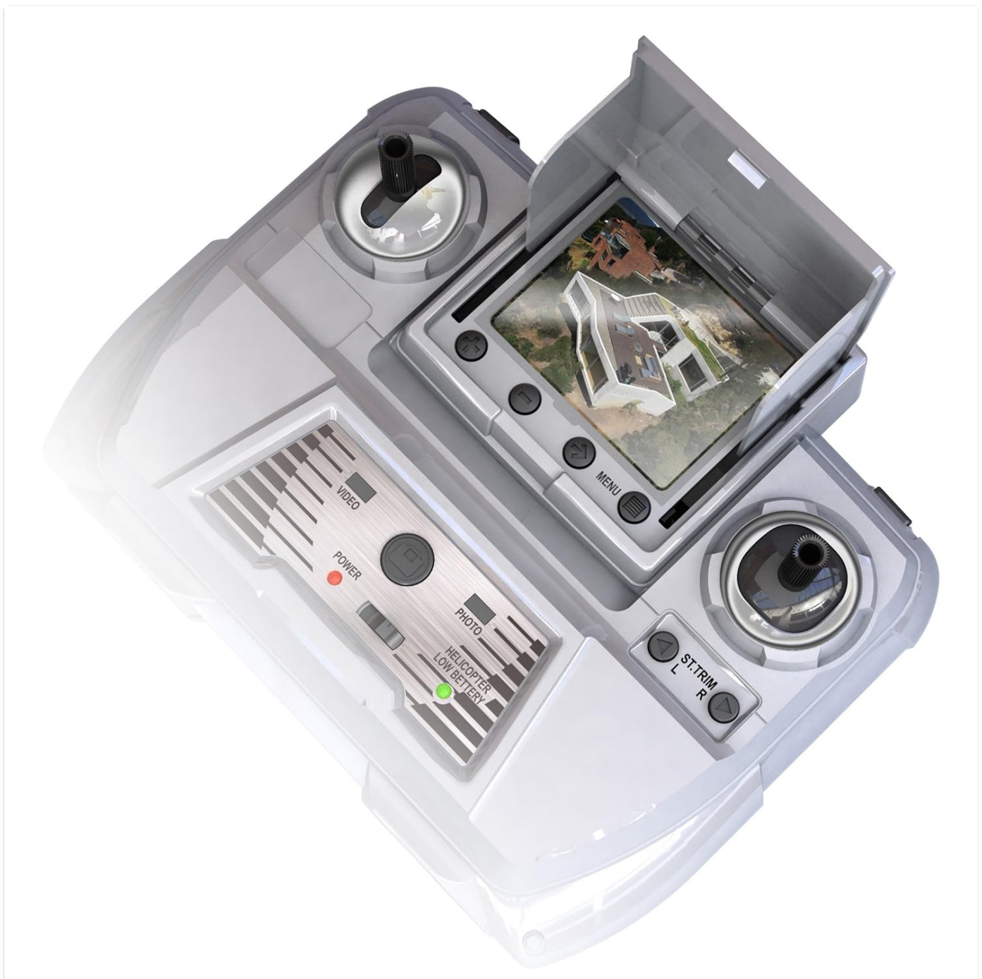
Figure 5.1: The transmitter displaying a live video feed from the helicopter's camera.
