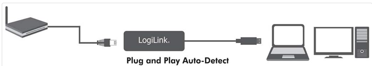
Image 5.2: The Logilink UA0144A adapter shown connected to a laptop, with an Ethernet cable plugged into its RJ45 port.
