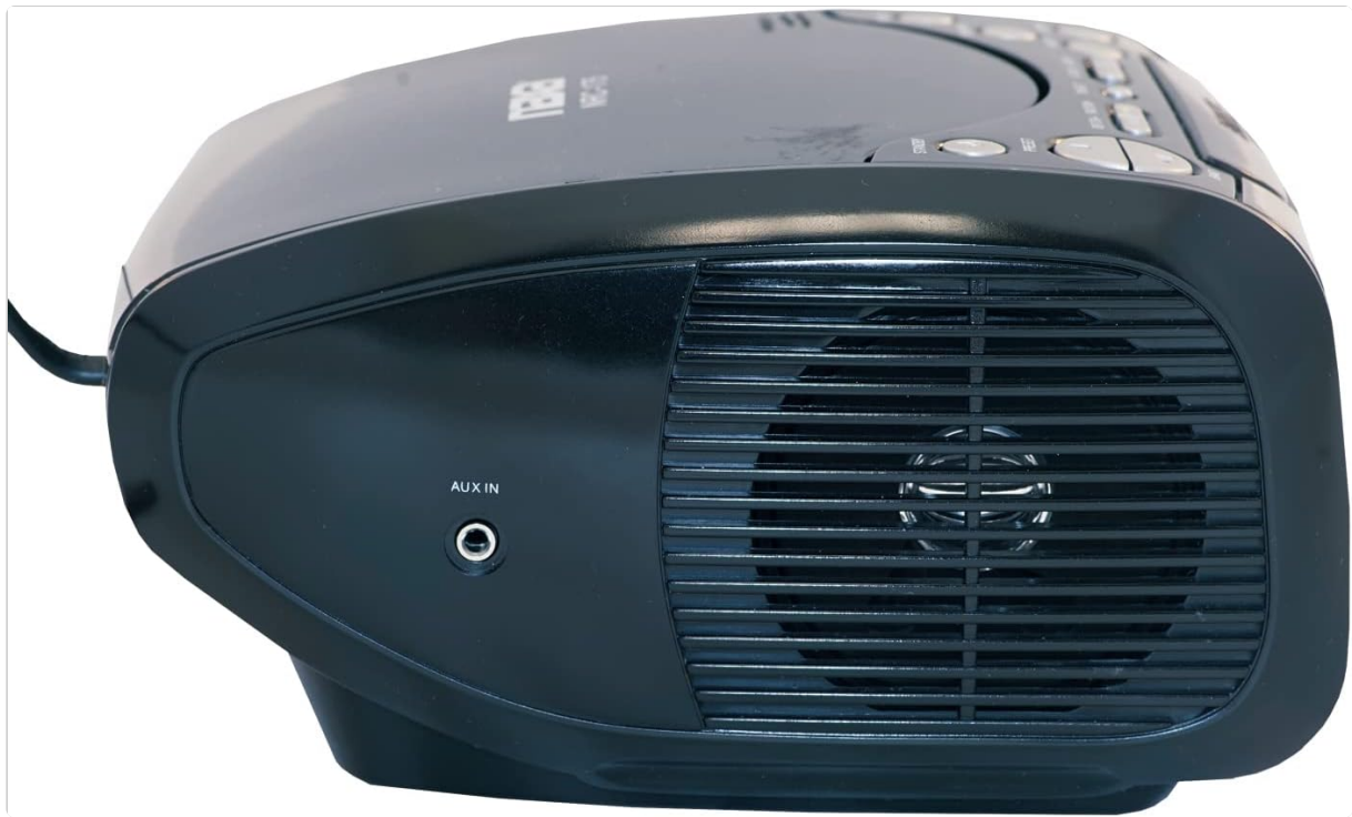
Figure 5.3: Side panel with AUX IN port.
