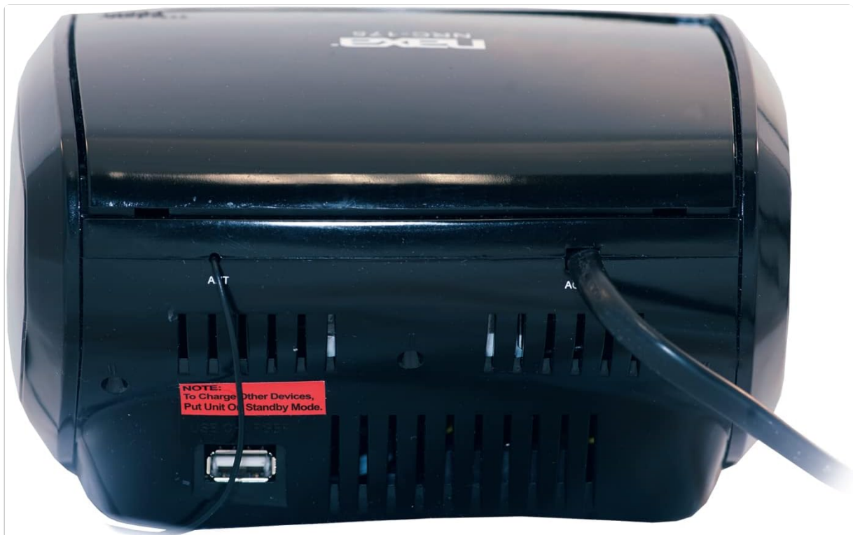
Figure 5.4: Rear panel with USB charging port and connections.
