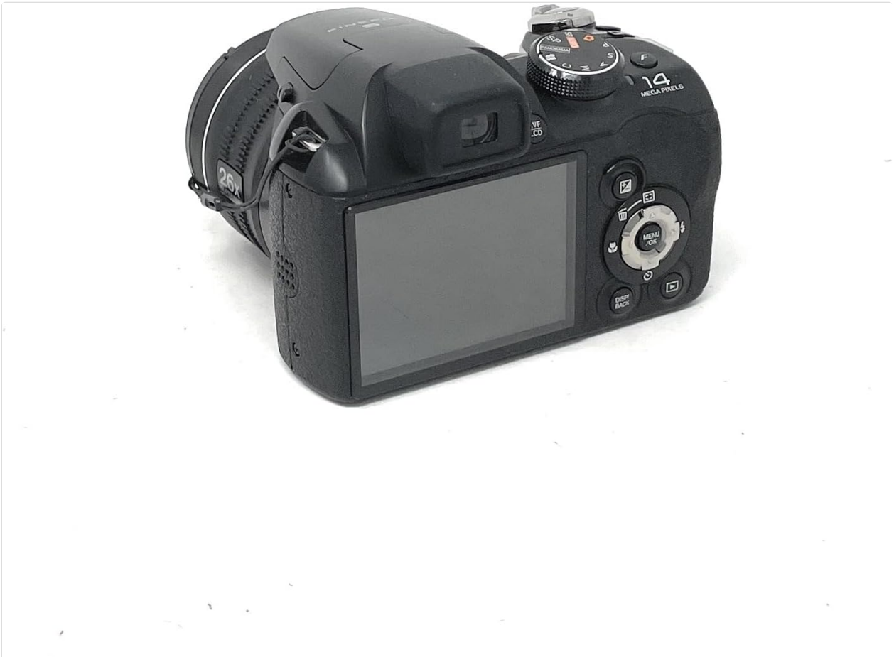
Figure 2: Rear view of the Fujifilm Finepix S4300 camera, displaying the 3-inch LCD screen and various
